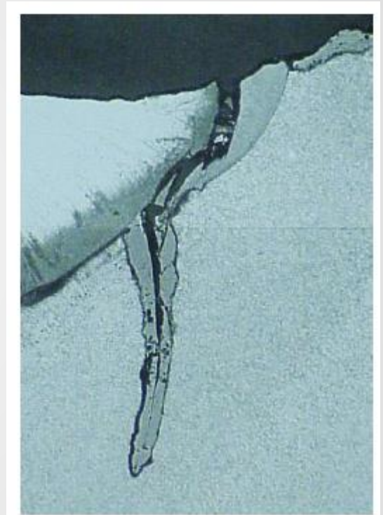
Superheater tube attachment fatigue cracking
