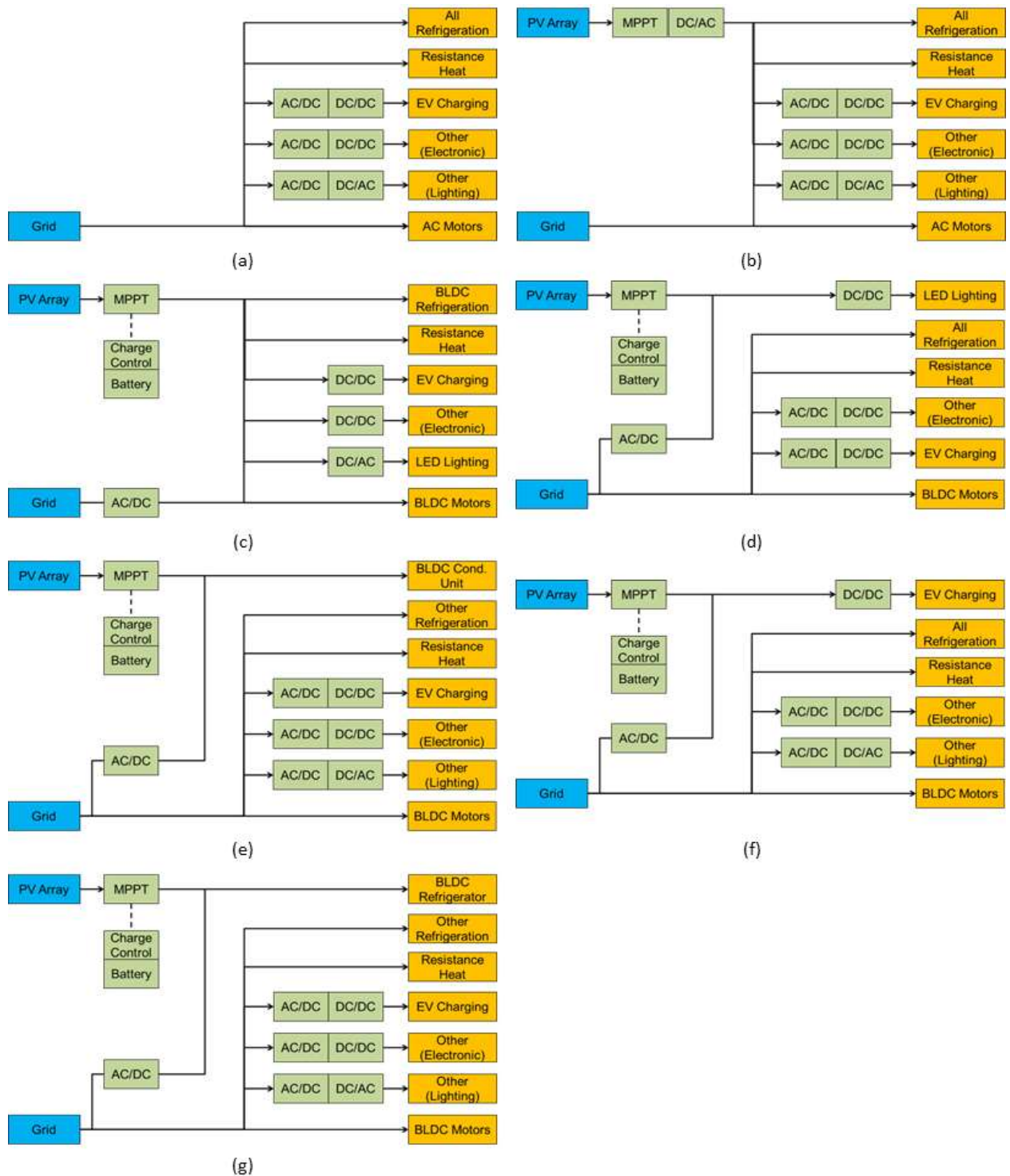
Figure 2. Schematic diagrams of simulated home configurations: (a) traditional home with AC distribution, without PV (b) traditional home with AC distribution and net-metered solar PV (c) home with DC distribution to all loads and net-metered PV with grid-rectified backup (d) home with DC distribution to a lighting circuit and net-metered PV with grid-rectified backup (e) home with DC distribution to a condensing unit and net-metered PV with grid-rectified backup (f) home with DC distribution to a PEV charger and net-metered PV with grid-rectified backup (g) home with DC distribution to a refrigerator and net-metered PV with grid-rectified backup.
